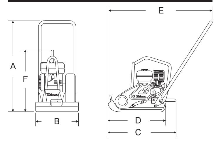
Figure 1. MVC-64H/HW Plate Compactor Dimensions
